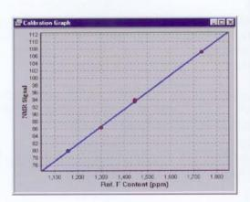
Calibration simply requires a minimum of six sodium fluoride standards (in distilled water) that span the concentrations of interest. The instrument is calibrated at installation and only requires ongoing calibration checks as a test of the performance.
